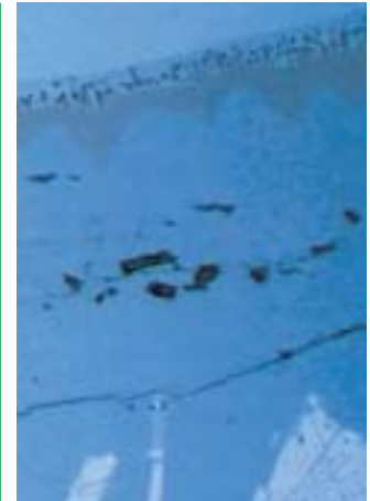
Glass body soldered into steel shell (500:1)
