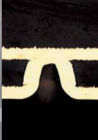
Circuit board with VIAS (500:1)
